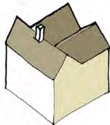
'M' Shaped Double Gable behind Standard Gable Roof: limited to farmhouses and later extensions
